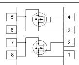
• 5.0 A, 30 V.  $R_{DS(ON)}$  = 0.050  $\Omega$  @  $V_{GS}$  = 10 V
