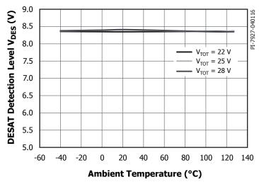
Figure 30. Desaturation Detection Level  $V_{DES}$  vs. Ambient Temperature. Conditions:  $V_{VCC} = 5 \text{ V}$ .
