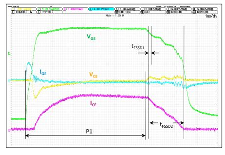
Figure 12. Advanced Soft Shut Down Function.
