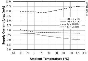
Figure 20. Supply Current Secondary-Side  $I_{\rm VISO}$  vs. Ambient Temperature. Conditions:  $V_{\rm VCC}=5$  V,  $V_{\rm TOT}=25$  V, No-Load.
