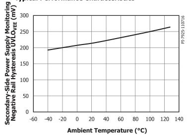
Figure 29. Power Supply Monitoring Negative Rail Hysteresis UVLO\_{VEE} vs. Ambient Temperature. Conditions:  $V_{VCC} = 5 \text{ V}$ .
