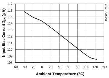
Figure 17. Input Bias Current vs. Ambient Temperature. Conditions:  $V_{\rm VCC} = 5$  V,  $V_{\rm IN} = 5$  V,  $V_{\rm TOT} = 25$  V.
