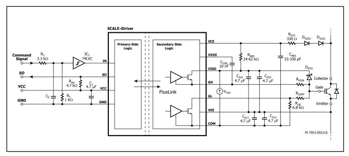
Figure 14. SCALE-iDriver Application Example Using Diodes for Desaturation Detection.
