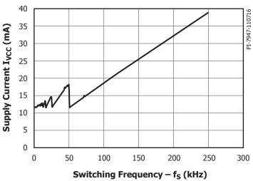
Figure 19. Supply Current Primary-Side  $I_{_{VCC}}$  vs. Switching Frequency. Conditions:  $V_{_{VCC}}=5$  V,  $V_{_{TOT}}=25$  V,  $T_{_{J}}=25$  °C, 0 Hz  $_{S}$   $_{S}$   $_{S}$   $_{S}$   $_{S}$   $_{S}$   $_{S}$   $_{S}$
