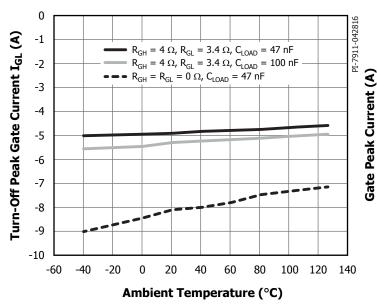
Figure 7. Turn-Off Peak Output Current (Sink) vs. Ambient Temperature. Conditions:  $V_{VCC} = 5 \text{ V}, V_{TOT} = 25 \text{ V}, f_{_S} = 20 \text{ kHz}, \text{Duty Cycle} = 50\%$
