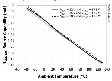
Figure 31. VEE Source Capability  $I_{\text{VEE(SO)}}$  vs. Ambient Temperature and  $V_{\text{VISO}}$ . Conditions:  $V_{\text{VCC}} = 5 \text{ V}$ ,  $f_{\text{S}} = 20 \text{ kHz}$ , Duty Cycle = 50%.
