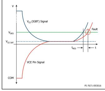
Figure 10. Short-Circuit Protection Using Rectifier Diode D<sub>vcr</sub>-
