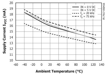
Figure 18. Supply Current Primary-Side  $I_{\rm VCC}$  vs. Ambient Temperature. Conditions:  $V_{\rm VCC}=5$  V,  $V_{\rm TOT}=25$  V, No-Load.
