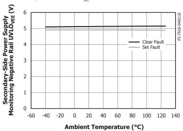
Figure 28. Power Supply Monitoring Negative Rail UVLO\_{\_{VEE}} vs. Ambient Temperature. Conditions:  $V_{_{VCC}} = 5 \ V$ .
