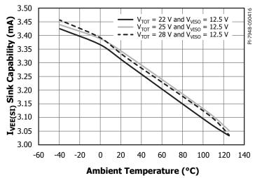
Figure 32. VEE Sink Capability  $I_{\rm VEE(SI)}$  vs. Ambient Temperature and  $V_{\rm VISO}$  Conditions:  $V_{\rm VCC}=5$  V,  $f_{\rm S}=20$  kHz, Duty Cycle = 50%.
