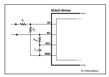
Figure 5. Increased Threshold Voltages  $V_{\mathit{IN+HT}}$  and  $V_{\mathit{IN+HT}}$  For  $R_{\scriptscriptstyle 1}=3.3~\mathrm{k}\Omega$  and  $R_{\scriptscriptstyle 2}=1~\mathrm{k}\Omega$  the IN Logic Level is 15 V.
