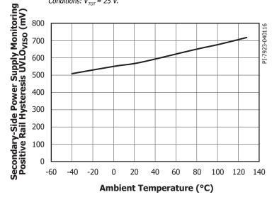
Figure 27 Power Supply Monitoring Positive Rail Hysteresis  $UVLO_{VISO}$  vs. Ambient Temperature. Conditions:  $V_{VCC} = 5 \ V$ .
