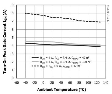
Figure 6. Turn-On Peak Output Current (Source) vs. Ambient Temperature. Conditions:  $V_{CC}=5~V,~V_{TOT}=25~V,~f_{_S}=20~kHz,~Duty~Cycle=50\%.$
