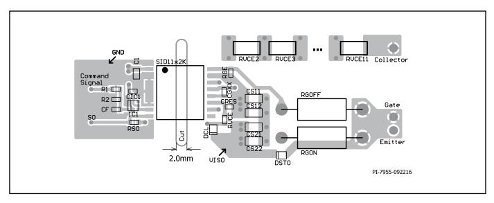
Figure 15a. Top View of Recommended PCB Layout. Corresponds to Schematic Shown in Figure 13.
