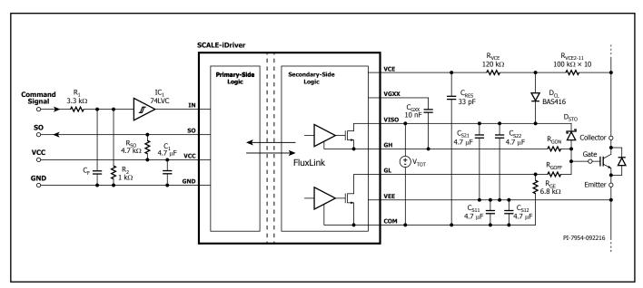
Figure 13. SCALE-iDriver Application Example Using a Resistor Network for Desaturation Detection.
