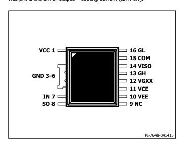
Figure 4. Pin Configuration.
