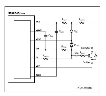
Figure 9. Short-Circuit Protection using a Resistor Chain  $R_{VCEX}$ .
