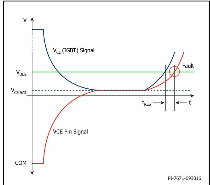
Figure 11. Short-Circuit Protection Using Resistors Chain  $R_{VCE}$
