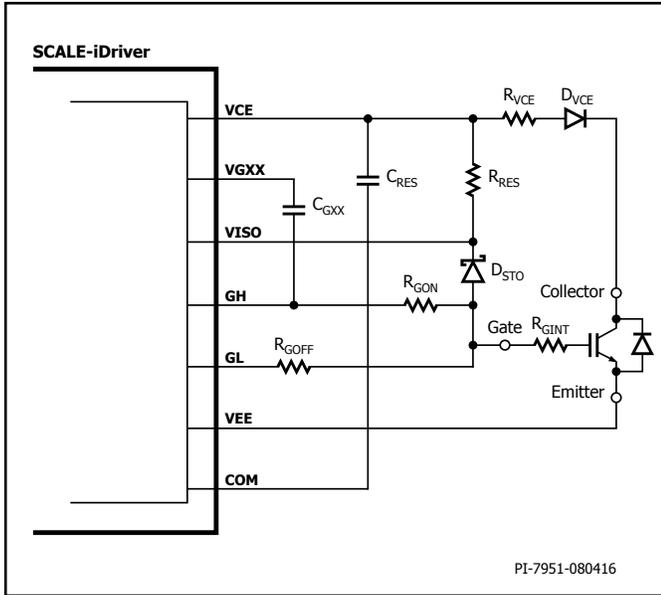
Figure 10. Short-Circuit Protection Using Rectifier Diode  $D_{VCE}$
