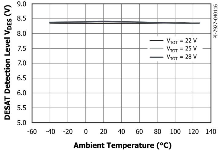
Figure 30. Desaturation Detection Level V<sub>DES</sub> vs. Ambient Temperature. Conditions: V<sub>VCC</sub> = 5 V.
