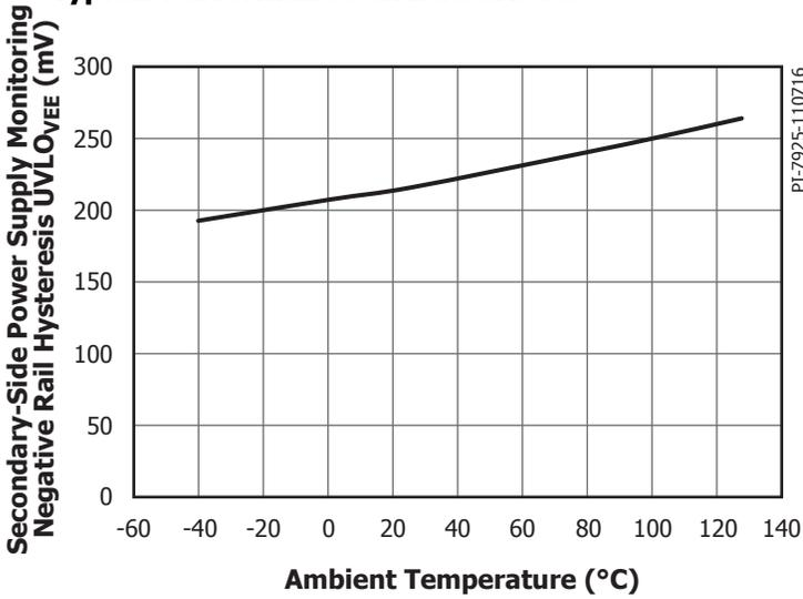
Figure 29. Power Supply Monitoring Negative Rail Hysteresis UVLO<sub>VEE</sub> vs. Ambient Temperature. Conditions: V<sub>VCC</sub> = 5 V.
