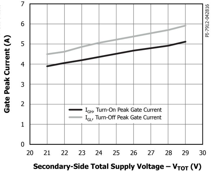
Figure 8. Turn-On and Turn-Off Peak Output Current vs. Secondary-Side Total Supply Voltage ( $V_{TOT}$ ). Conditions:  $V_{VCC} = 5\text{ V}$ ,  $T_j = 25\text{ °C}$ ,  $R_{GH} = 4\text{ Ω}$ ,  $R_{GL} = 3.4\text{ Ω}$ ,  $C_{LOAD} = 100\text{ nF}$ ,  $f_s = 1\text{ kHz}$ , Duty Cycle = 50%.
