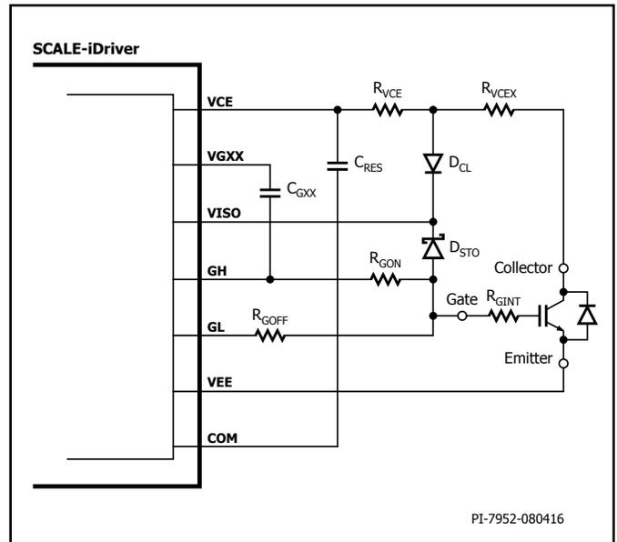
Figure 9. Short-Circuit Protection using a Resistor Chain  $R_{VCEX}$
