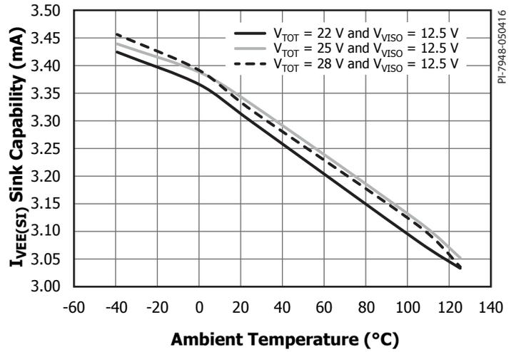
Figure 32. VEE Sink Capability I<sub>VEE(SI)</sub> vs. Ambient Temperature and V<sub>VISO</sub>. Conditions: V<sub>VCC</sub> = 5 V, f<sub>s</sub> = 20 kHz, Duty Cycle = 50%.
