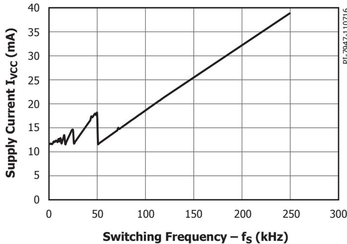
Figure 19. Supply Current Primary-Side  $I_{VCC}$  vs. Switching Frequency. Conditions:  $V_{VCC} = 5\text{ V}$ ,  $V_{TOT} = 25\text{ V}$ ,  $T_J = 25\text{ }^\circ\text{C}$ ,  $0\text{ Hz} \leq f_S \leq 250\text{ kHz}$ , No-Load.
