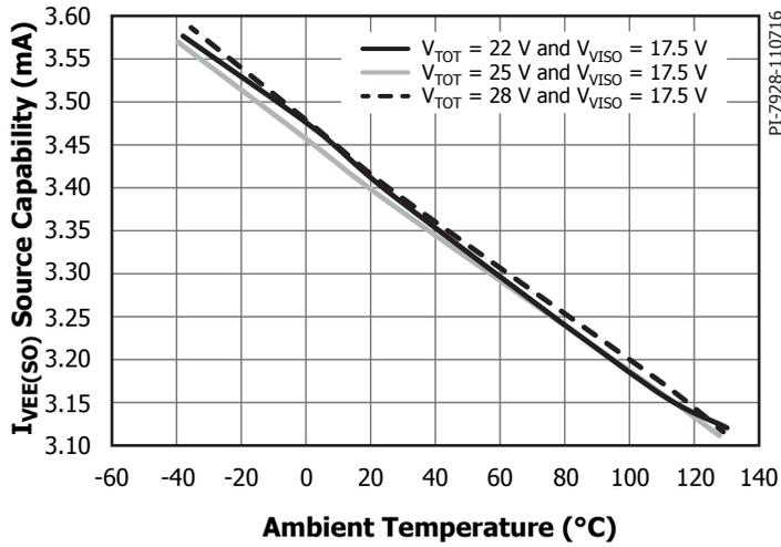
Figure 31. VEE Source Capability I<sub>VEE(SO)</sub> vs. Ambient Temperature and V<sub>VISO</sub>. Conditions: V<sub>VCC</sub> = 5 V, f<sub>s</sub> = 20 kHz, Duty Cycle = 50%.
