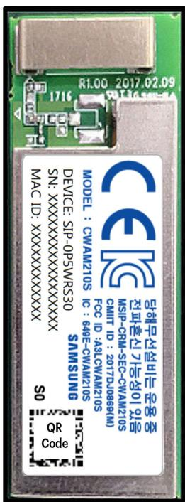
Figure 1. ARTIK 053s Module Top View
