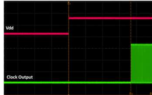
Figure 17. Startup Waveform vs. Vdd
