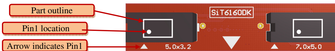
Figure 2: Time Machine socket card SiT6160DK. Supports 5.0mm x 3.2mm (6-pin) and 7.0mm x 5.0mm (6-pin)
