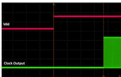
Figure 17. Startup Waveform vs. Vdd
