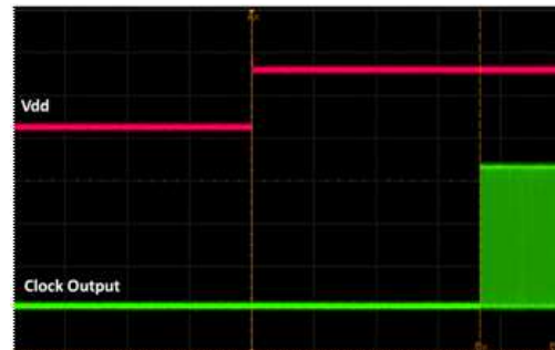
Figure 16. Startup Waveform vs. Vdd
