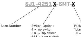
5RS = ring switch 6 = tip and ring switch Package Options "blank" = standard TR = Tape & Reel
