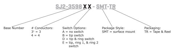
Note: 1. 3 conductor option only available with tip & ring switch
