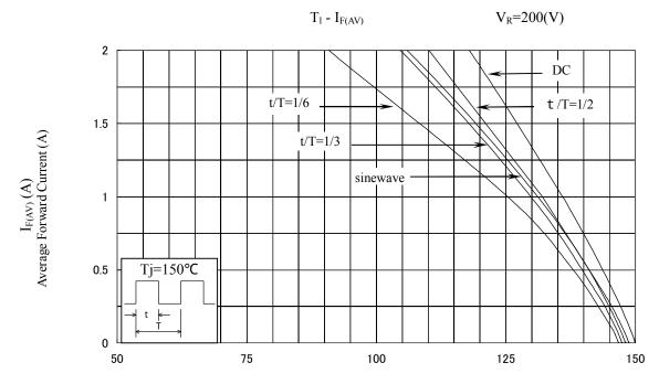
$\begin{array}{c} T_1\left(^{\circ}C\right) \\ \text{Lead Temperature}\left(^{\circ}C\right) \end{array}$
