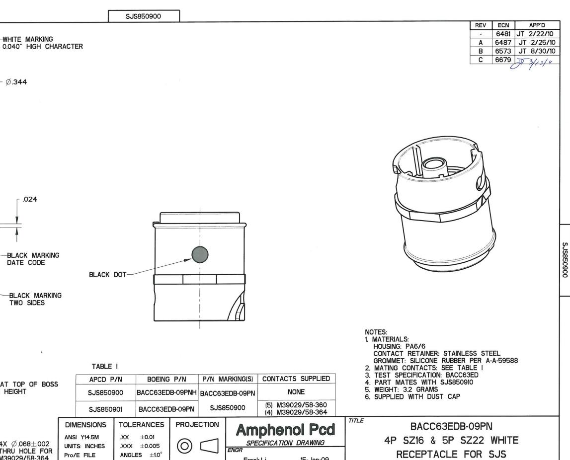
$\emptyset.672$ Ø.344 3X 30° Ø.410 3X 60°  $\emptyset.651$  $\emptyset$ .553 .077 .024 BACC63EDB-09PN SJS850900 APCD YYWW BLACK MARKING SJS850900 DATE CODE .678 BLACK MARKING TWO SIDES  $\emptyset.630$ Ø.180 AT BASE Ø.176 AT TOP OF BOSS X .265 HEIGHT
