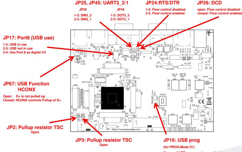
Open: UART programming enabled Closed: USB programming enabled
