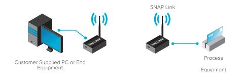
One SNAP Link Adaptor controls multiple SNAP Link serial wireless adapters (either RS-232 or RS-485/422).
