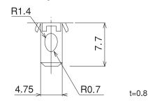
Solder Terminal (It can be used for TAB #187)
