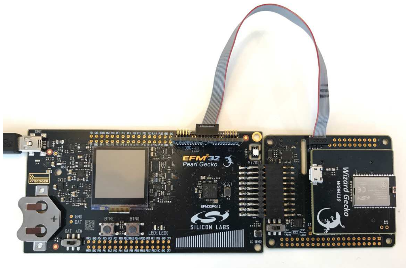
Figure 5.1. MCU Starter Kit as Programmer for WGM110 Wi-Fi Module Radio Board
