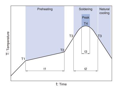
Soldering Preheating Peak Temp. Temp. Time Time Temp. Time T1 T2 T4 Т3 t3 150°C 180°C 60 to 120s 230°C 250°C 30s 5s
