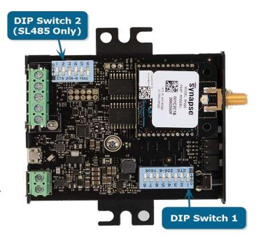
To access the DIP switches, remove the screw adjacent to the serial connection (DE-9 connector or terminal block) and lift the top of the enclosure off to expose the switches.
