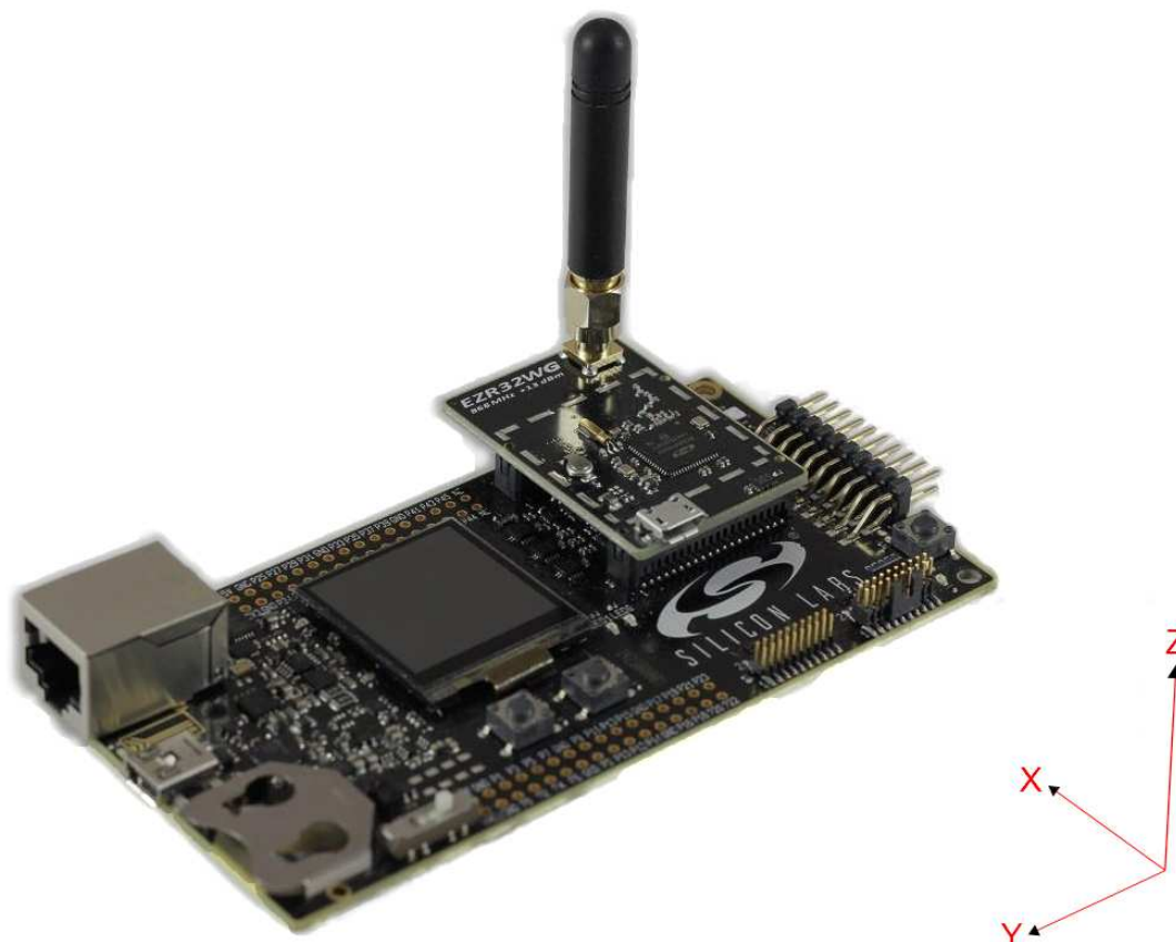
Figure 6.2. DUT: BRD4502A (Rev. B00) Radio Board with Wireless Starter Kit Mainboard
