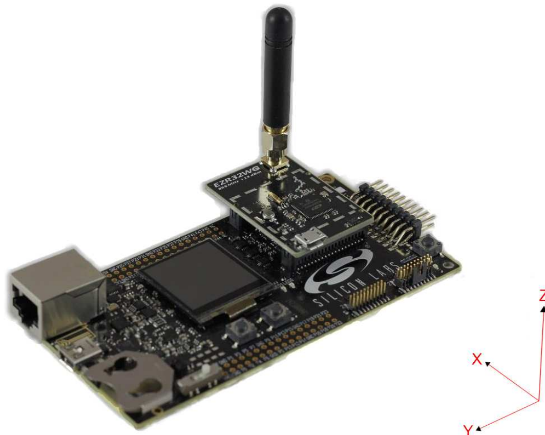
Figure 6.2. DUT: BRD4502D (Rev. A00) Radio Board with Wireless Starter Kit Mainboard
