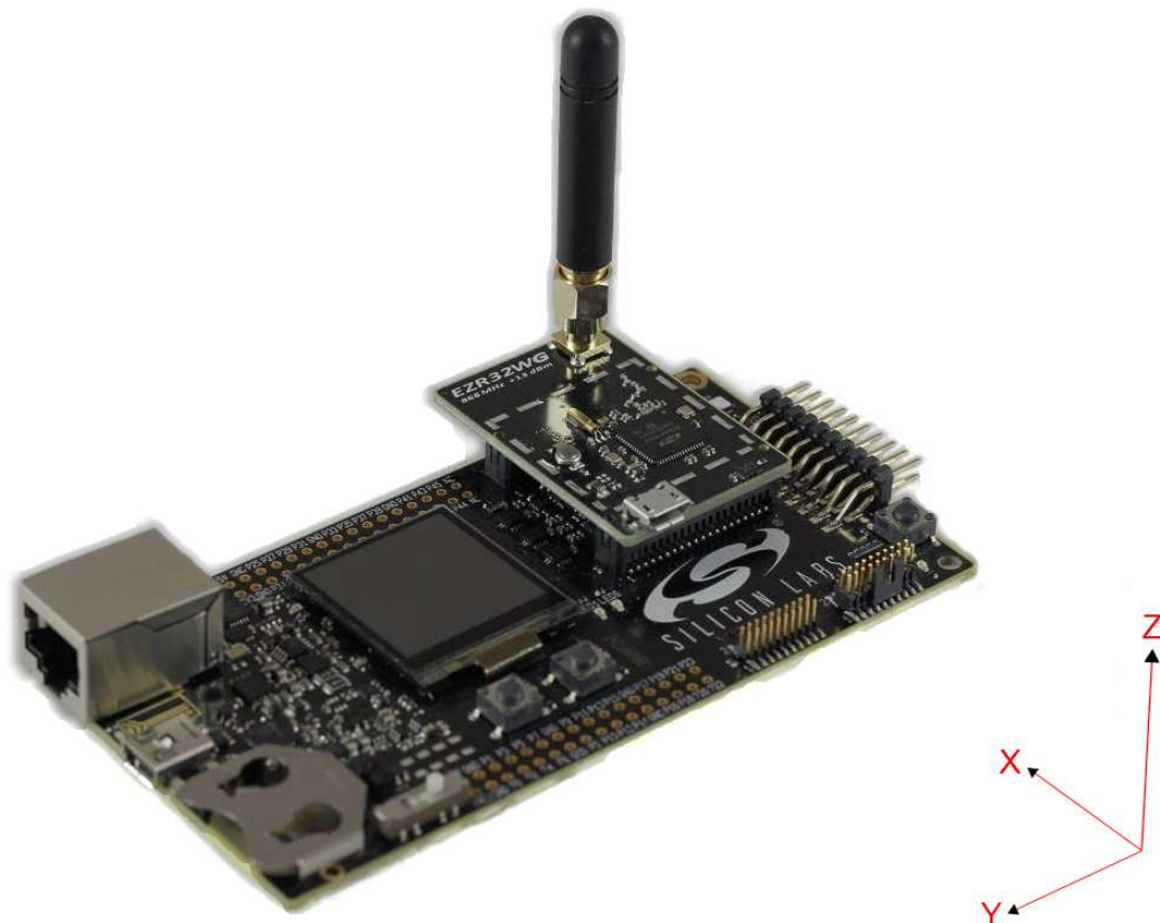
Figure 6.2. DUT: BRD4503A (Rev. B00) Radio Board with Wireless Starter Kit Mainboard
