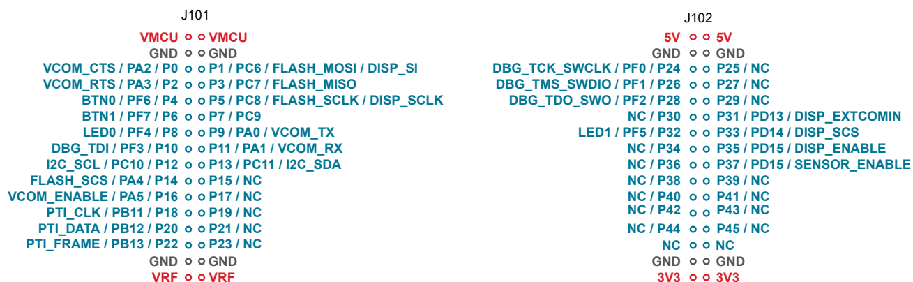
Figure 4.2. Radio Board Pin Mapping on Breakout Pads
