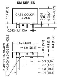
DIMENSIONS: INCHES (MILLIMETERS) TOLERANCE: ±0.020 (±0,50)
