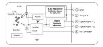
P1: small particle (1 ~  $2\mu$ m), P2: large particle (3 ~ $10\mu$ m)
