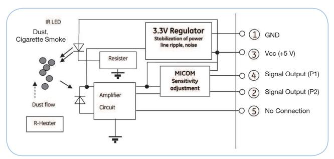
P1: small particle (1~ 2μm), P2: large particle (3~10μm)
