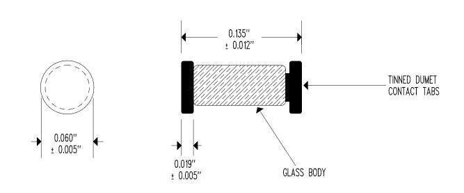
RESISTANCE @  $+25^{\circ}$ C = 1,000  $\Omega$  ± 10% RESISTANCE/TEMPERATURE CURVE = "E" BETA " $\beta$ " (0 TO  $+50^{\circ}$ C) = 3,263 K NOMINAL BETA " $\beta$ " (+25 TO  $+85^{\circ}$ C) = 3,347 K NOMINAL TEMPERATURE COEFFICIENT @  $+25^{\circ}$ C = -3.67%/C NOMINAL DISSIPATION CONSTANT = 2 mW/C NOMINAL THERMAL TIME CONSTANT = 8 SECONDS NOMINAL MAXIMUM TEMPERATURE RATING =  $+220^{\circ}$ C
