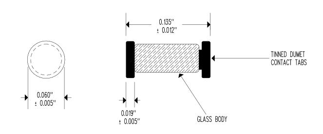
RESISTANCE @  $+25^{\circ}C = 10,000 \Omega \pm 10\%$ RESISTANCE/TEMPERATURE CURVE = "J" BETA " $\beta$ " (0 TO  $+50^{\circ}C$ ) = 3,892 $^{\circ}K$  NOMINAL TEMPERATURE COEFFICIENT @ +25C = -4.4% $^{\circ}C$  NOMINAL DISSIPATION CONSTANT = 2 mW/ $^{\circ}C$  NOMINAL THERMAL TIME CONSTANT = 8 SECONDS NOMINAL MAXIMUM TEMPERATURE RATING =  $+220^{\circ}C$
