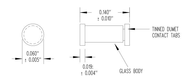
RESISTANCE @  $+25^{\circ}\text{C} = 100,000 \ \Omega \pm 1\%$ RESISTANCE/TEMPERATURE CURVE = "J" BETA " $\beta$ " (0 TO  $+50^{\circ}\text{C}$ ) = 3,892°K NOMINAL TEMPERATURE COEFFICIENT @  $+25^{\circ}\text{C} = -4.4\%$ /°C NOMINAL DISSIPATION CONSTANT = 2 mW/°C NOMINAL (STILL AIR) MAXIMUM OPERATING TEMPERATURE =  $+220^{\circ}\text{C}$
