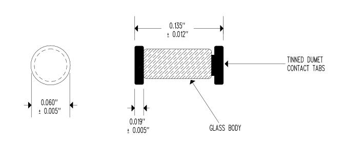
RESISTANCE @ +25'C =  $2,186 \Omega \pm 10\%$ RESISTANCE/TEMPERATURE CURVE = "E1" BETA " $\beta$ " (0 TO +50'C) = 3,320'K NOMINAL TEMPERATURE COEFFICIENT @ +25'C = -3.82%/'C NOMINAL DISSIPATION CONSTANT = 2 mW/'C NOMINAL THERMAL TIME CONSTANT = 8 SECONDS MAXIMUMMAXIMUM TEMPERATURE RATING = +220'C
