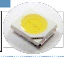
Bivar Surface Mount 3527 package LED may be used in nearly any lighting or backlighting application. These 0.1 Watt SMD LED's have a minimum CRI Value of 80 and are available in 3 color temperatures to meet any illumination needs: Cool, Neutral and Warm White. The SM3527 Series is conveniently packaged in standard tape and reels for pick and place assemblies.
