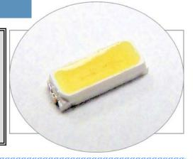
Bivar Surface Mount 4014 package LED may be used in nearly any lighting or backlighting application. These 0.2 Watt SMD LED's have a minimum CRI Value of 80 and are available in 3 color temperatures to meet any illumination needs: Cool, Neutral and Warm White. The SM4014 Series is conveniently packaged in standard tape and reels for pick and place assemblies.
