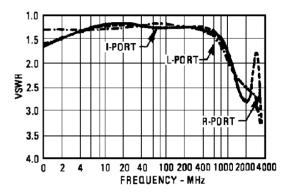
VSWR vs. Frequency: VSWR is the L-, l-, and R-ports in a 50 ohm system with  $f_L$  at +10 dBm. R- and I-port VSWR plotted with  $f_L$  at 1500 MHz.
