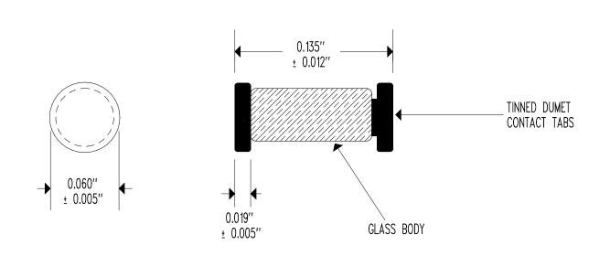
RESISTANCE @  $+25^{\circ}$ C =  $500 \Omega \pm 10^{\circ}$ RESISTANCE/TEMPERATURE CURVE = "B" BETA " $\beta$ " (0 TO  $+50^{\circ}$ C) =  $2,941^{\circ}$ K NOMINAL TEMPERATURE COEFFICIENT @  $+25^{\circ}$ C =  $-3.31^{\circ}$ / $^{\circ}$ C NOMINAL DISSIPATION CONSTANT =  $2 \text{ mW/}^{\circ}$ C NOMINAL THERMAL TIME CONSTANT = 8 SECONDS NOMINALMAXIMUM TEMPERATURE RATING =  $+220^{\circ}$ C
