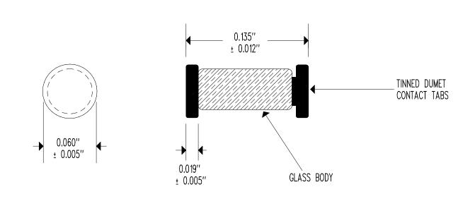
RESISTANCE @  $+25^{\circ}C$  =  $500,000 \Omega$   $\pm$   $10^{\circ}$  RESISTANCE/TEMPERATURE CURVE = "R" BETA " $\beta$ " (0 TO  $+50^{\circ}C$ ) =  $4,140^{\circ}K$  NOMINAL TEMPERATURE COEFFICIENT @  $+25^{\circ}C$  =  $-4.68^{\circ}/^{\circ}C$  NOMINAL DISSIPATION CONSTANT = 2 mW/ $^{\circ}C$  NOMINAL THERMAL TIME CONSTANT = 8 SECONDS MAXIMUM MAXIMUM TEMPERATURE RATING =  $+220^{\circ}C$
