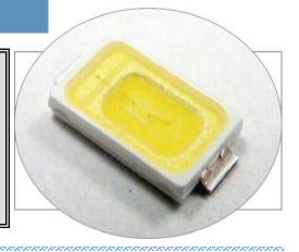
Bivar Surface Mount 5730 package LED may be used in nearly any lighting or backlighting application. These 0.5 Watt SMD LED's have a minimum CRI Value of 80 and are available in 3 color temperatures to meet any illumination needs: Cool, Neutral and Warm White. The SM5730 Series is conveniently packaged in standard tape and reels for pick and place assemblies.
