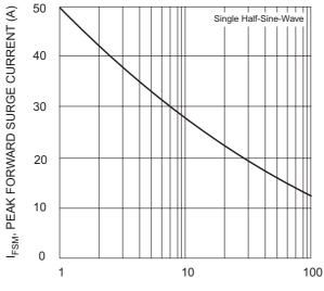
NUMBER OF CYCLES AT 60 Hz Fig. 2 Max Non-Repetitive Peak Forward Surge Current
