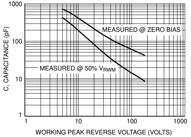
Figure 8. Capacitance versus Working Peak Reverse Voltage
