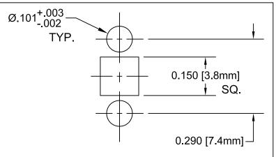
Recommended Soldering Pattern & Mounting Holes
