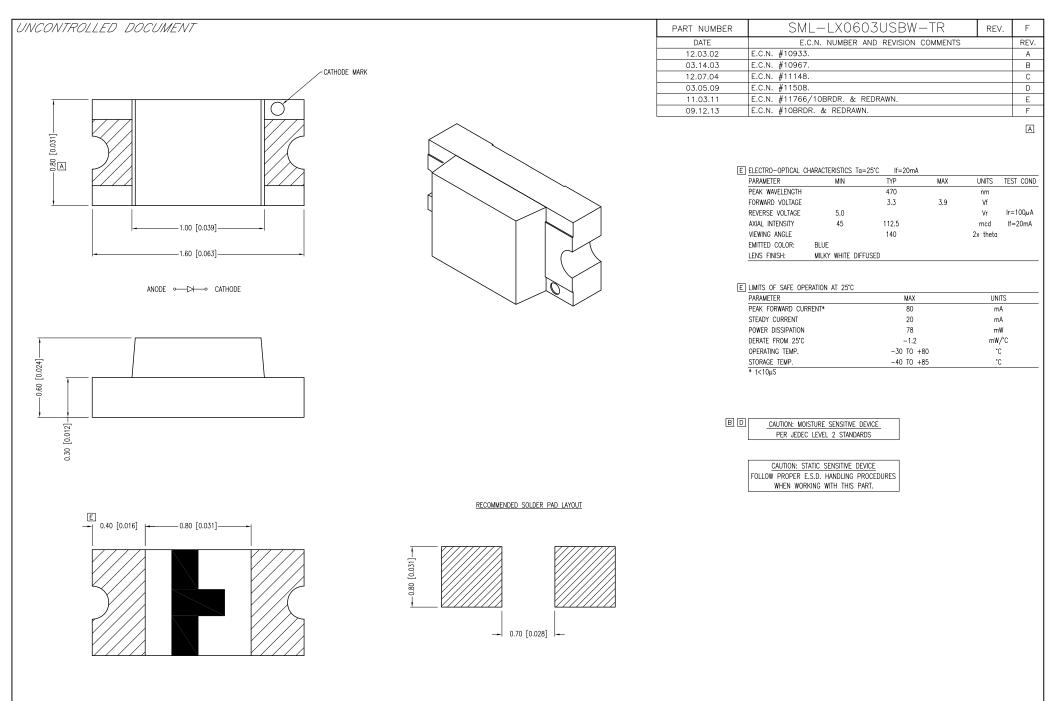
\*UNLESS OTHERWISE SPECIFIED TOLERANCES PER DECIMAL PRECISION ARE: X=±1 (±0.039), X.X=±0.5 (±0.020), X.XX=±0.25 (±0.010), X.XXX=±0.127 (±0.005). LEAD SIZE=±0.05 (±0.002), LEAD LENGTH=±0.75 (±0.030). MIN=  $\frac{+DECIMAL}{-0.00}$  MAX.=  $\frac{+0.00}{-0.00}$
