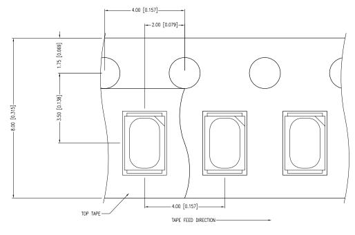
\*UNLESS OTHERWISE SPECIFIED TOLERANCES PER DECIMAL PRECISION ARE: X=±1 (±0.039), X.X=±0.5 (±0.020), X.XX=±0.25 (±0.010), X.XXX=±0.127 (±0.005). LEAD SIZE=±0.05 (±0.002), LEAD LENGTH=±0.75 (±0.030). MIN=  $^{+0.00}_{-0.00}$  MAX.=  $^{+0.00}_{-0.00}$  MAX.=  $^{+0.00}_{-0.00}$  MAX.=  $^{+0.00}_{-0.00}$  PRECISION UNCONTROLLED DOCUMENT
