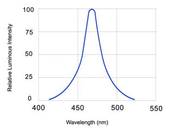
Fig.1 Relative Luminous Intensity vs. Wavelength
