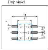
Terminal (E) to be connected to Ground. Terminal (E) is connected to the metal frame.
