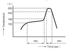
Apply reflow soldering only once
