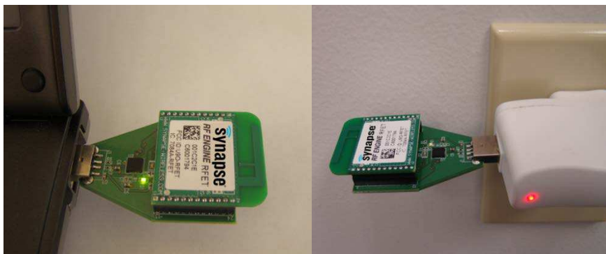
Figure 3 – A SNAPstick drawing power from a laptop PC and USB AC Adapter
