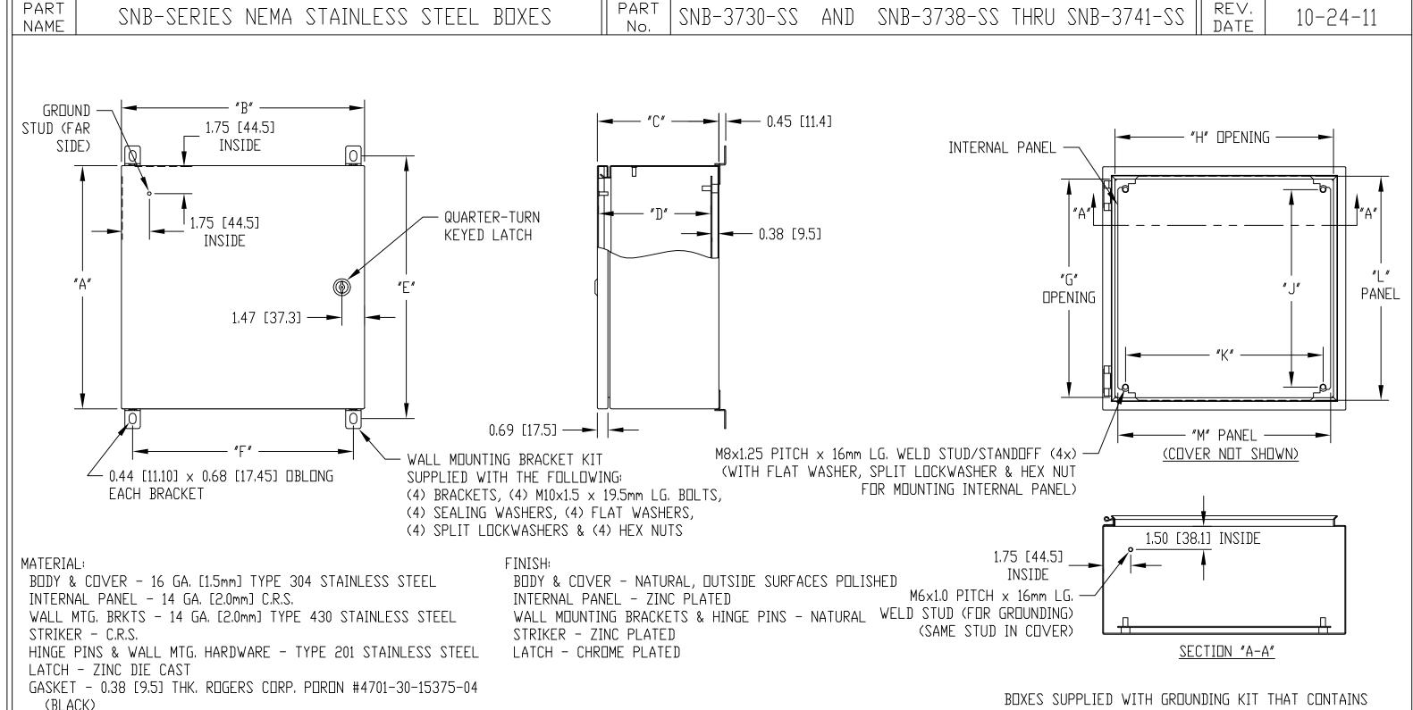
BUXES SUPPLIED WITH GROUNDING KIT THAT CONTAINS THE FOLLOWING: (1) GROUND WIRE, (4) FLAT WASHERS, (2) SPLIT LOCKWASHERS AND (2) HEX NUTS
