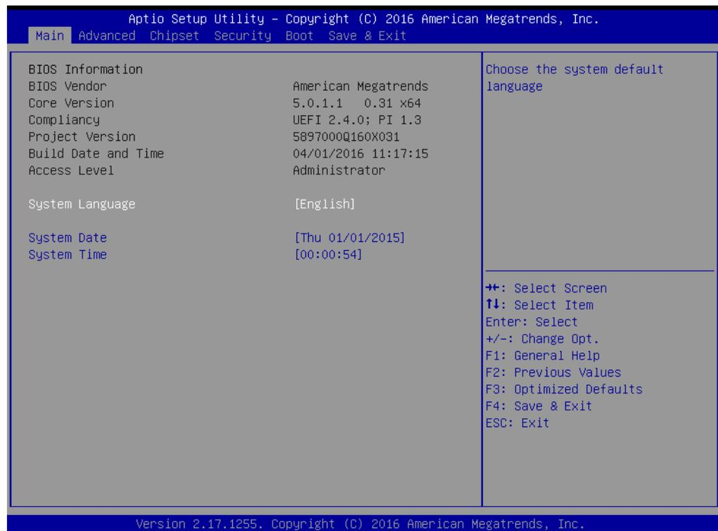
The BIOS setup screen has three main frames. The left frame displays all information and configurable items. Grayed-out text is information only. Blue items are options that can be configured. White one is the current focus item to be selected.
