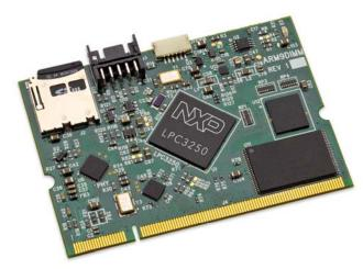
Modular LPC3250 based Microprocessor Plug-In System On Module
