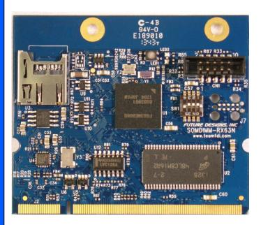
Modular RX63N based Microcontroller Plug-In System-On-Module
