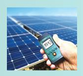
Extech's SP505 measures solar power level from outdoor sunlight to determine the best location of solar panel and solar water heater installations. It is also used indoors by window manufacturers, automotive industry, and remodeling home owners to check the level of solar radiation transmission through various glass thicknesses and degrees of tinting to use for window installations. Convenient pocket-sized meter with built-in precision solar light sensor is easy-to-use wherever you go.
