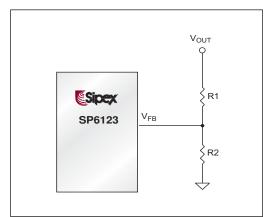
Figure 5. A voltage divider connected to the  $V_{FB}$  pin programs the output voltage.
