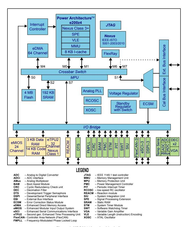
Figure 1. MPC5644A series block diagram
